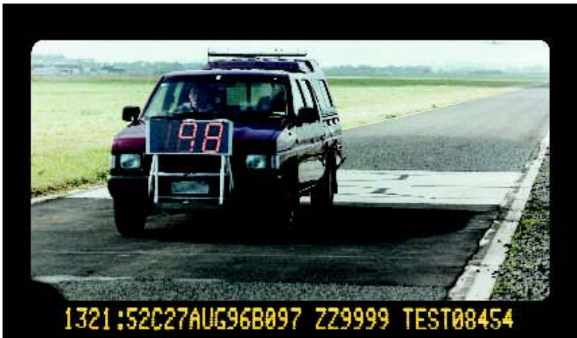
Figure 21 Calibrating a Speed Camera
